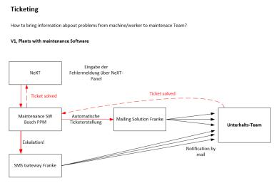
Ticket handling will be done from "maintenance software". Also counting for open tickets/costcenter should be done at "maintenance software", but result has to be delivered to "NeXT" for displaying result.
