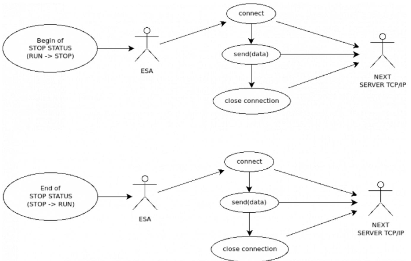
Considering a STOP event for one of the two robots, it is necessary to send the 2 messages in a specific order, in particular:
