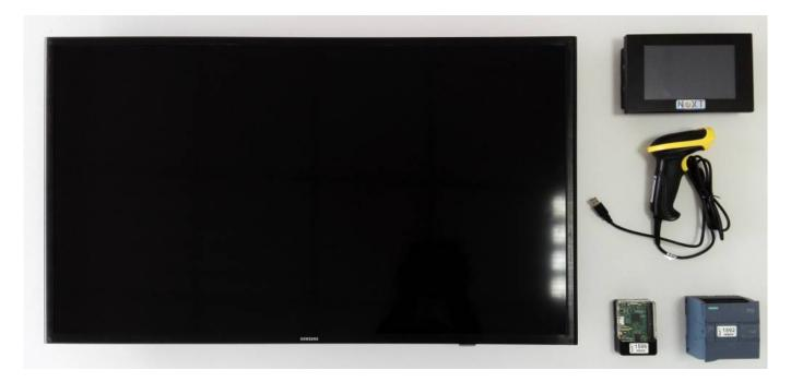
Connected to the touch panel is the barcode reader that will help the operator **change the production order** and, in case of absence of the PLC, **increase the number of pieces produced**.
