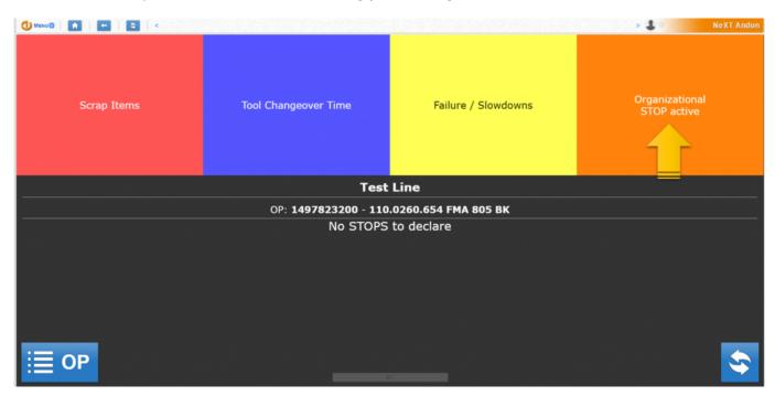
• Press the blinking area to end the stop machine. The system will ask for confirmation
