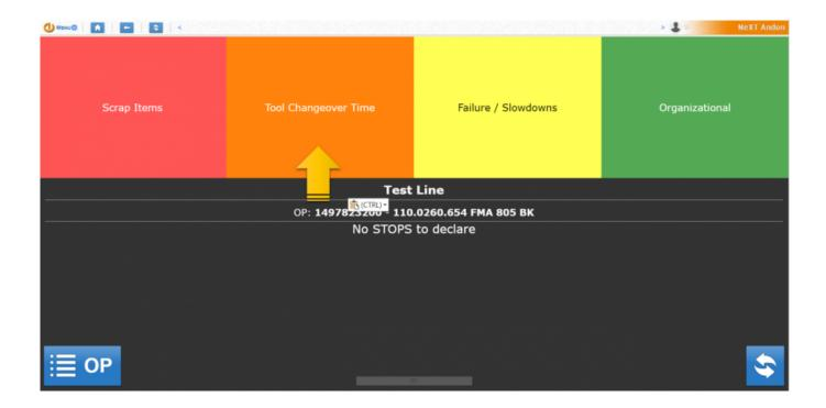
• Press the blinking area to end the tooling. The system will ask for confirmation.
