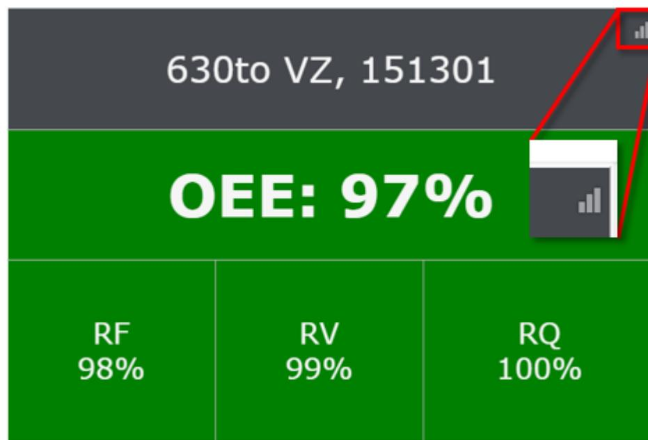
The following image shows the OEE interface. By default, it shows the OEE value of the current day, hour by hour, starting from the beginning of the shift.
