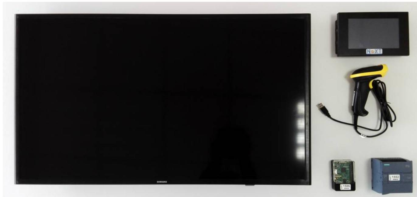
The barcode reader connected to the touch panel will help the operator **change the production order** and, in case the PLC is missing, to **increase the number of pieces produced**.
