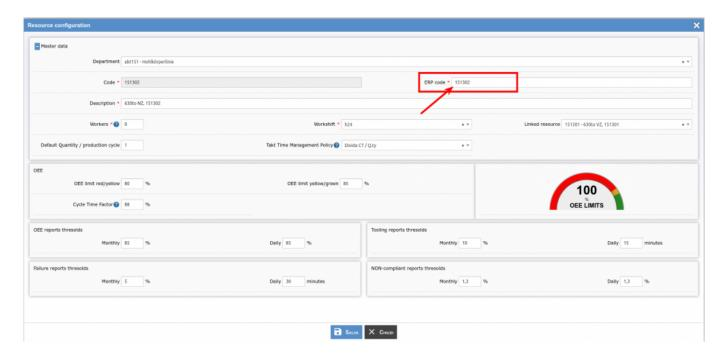
For the case of work-center it is necessary to check if GEC platform will use the same code of the SAP system. If YES, no additional operation will be required since IMPROVE 4.0 is already configured for this scope. If NOT, it will be necessary to add another field in the same page for mapping the GEC platform work centers codes.
